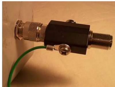
replaceable element, to access it remove the screw on the side of the arrestor. The total installed cost of Yagi antennas including the cable, surge arrestor, pole (if needed), time and labor required etc. is usually insignificant between the
