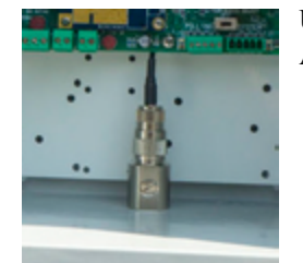
External Antenna with Surge Arrester
